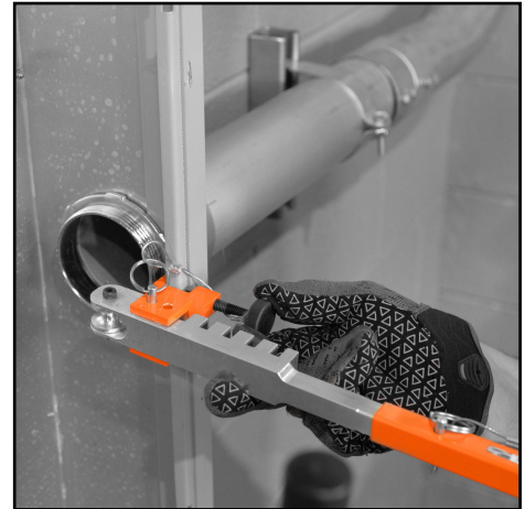
Head Captures Edge of Panel Box
