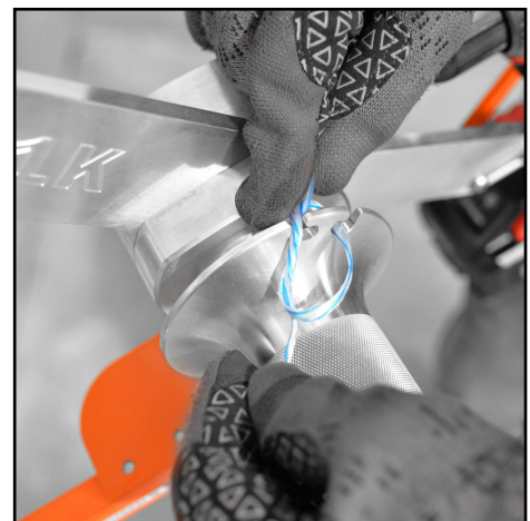
Capstan Cleat Captures Rope or String
