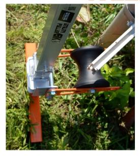
Step 9. When ready begin, thread rope tale over the rope engagement roller and pull up on in a steady continuous motion to start the pull.
