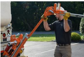
Step 4.1 Insert the lower extension and roller.
