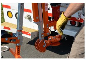
Step 7.1 Align front arm be in line with the direction of the pull.
