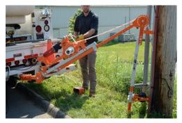
Step 10. Press forward/ reverse button to center position to put in neutral.
