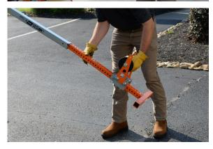
Step 4.2 Tip puller to upright and collapsed position and replace all pins.
