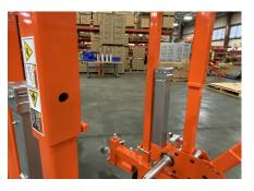
3.) Insert 5/8"Bolts on both sides, tighten.
