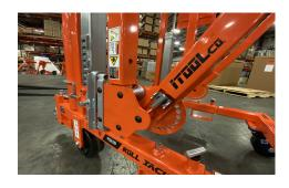
2.) Using a forklift, raise the cross member until the two bolt holes positioned on the sides of the sliding arms are aligned.
