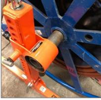
Axle-less on steel reel with 2" arbor holes
