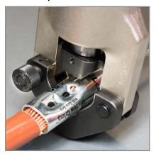
2. Use a 12 ton die crimping tool to squeeze the head in one or two positions.
