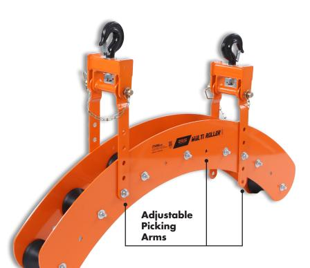
The Multi Roller features extra wide, profiled phenolic rollers. Rollers ride on rated bearings. Extra deep side walls (made from 1/4" 6061 aluminum) offer a light yet durable tool. The adjustable picking arms allow users to fine tune the adjustment angle without extra rigging.
