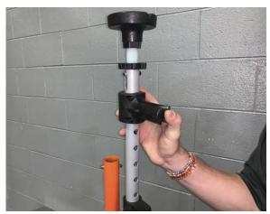
Step 7: To add extension, remove rubber retaining rings from the two fastened positions as seen here.
