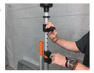
Step 6: While pulling down on gas shock engagement handle, use thumb or finger to engage gas shock with pressure on handle adjust to your working height.
