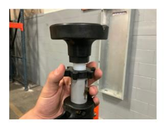
To lock and unlock pull and turn 90 degree as shown here. Note vertical positioning is locked.
