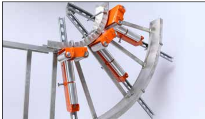
Cable and wire turn corners smoothly.
